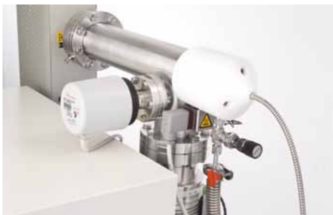
HPR-20 QIC TMS transient MS QIC inlet
